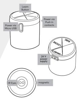
Be aware of the correct positioning of the connectors on the power meter.
